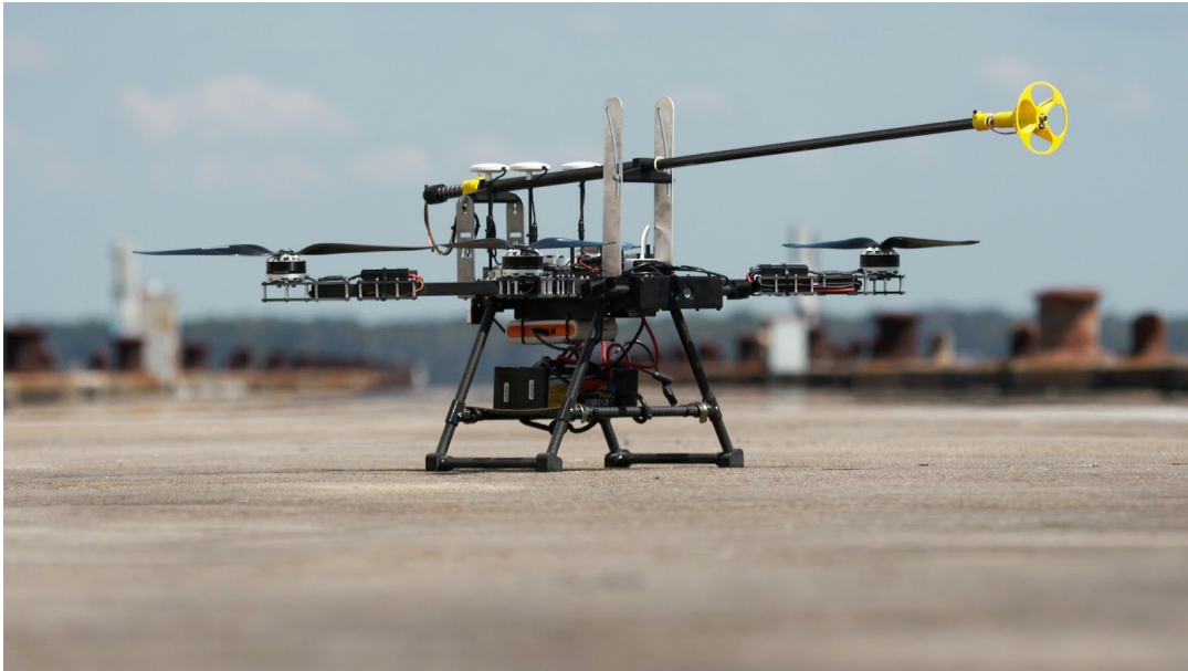
Figure 1: Apellix NDT Aerial Robot
