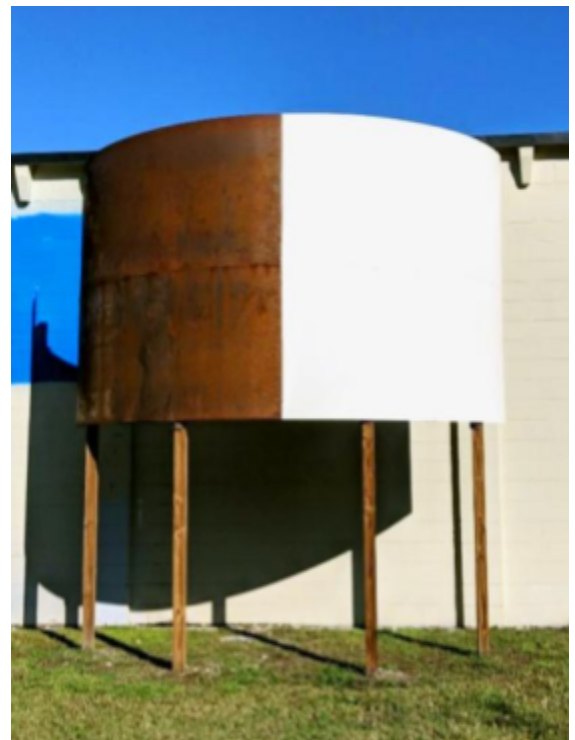
Figure 2: Coated and Uncoated Elevated Carbon Steel Test Plates
